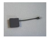
The barometric pressure smart sensor is designed to work with HOBO® stations. The smart sensor has a plug-in modular connector that allows it to be added easily to a HOBO station. All calibration parameters are stored inside the smart sensor, which automatically communicates configuration information to the logger without any programming or extensive user setup.
