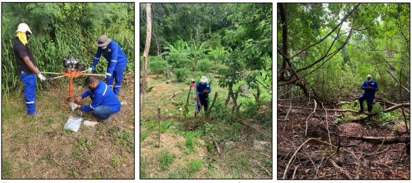
Selected Fieldwork Photos: Auger Drilling and Sampling (left image), Topographic Surveying (middle image) and GPS Line Transects (right image).
