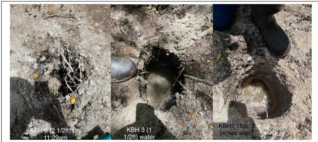
Soil Sample 6 (KBH6)- Auguring and Sampling. - Water Table/Hydraulic head measurements
