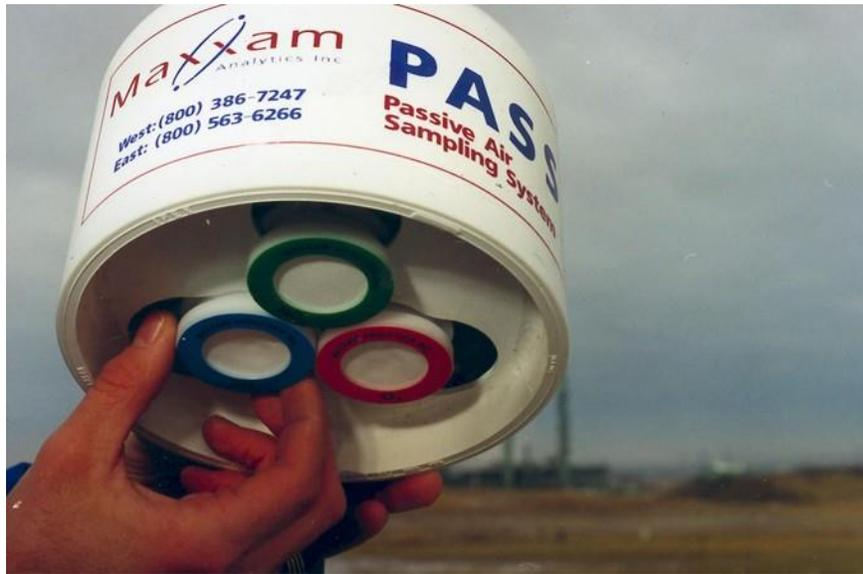
**FIGURE 1.** Passive samplers of Maxxam all-season passive sampling system.
