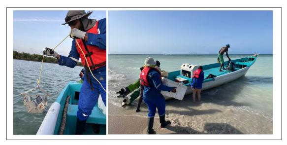
Marine Sediment Sampling KBMS-1 and 3 with Ponar grab sampler.
