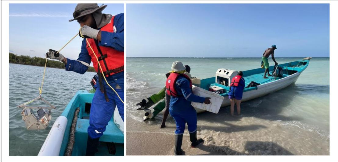
Marine Sediment Sampling KBMS-1 and 3 with Ponar grab sampler.
