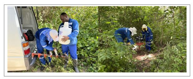
Soil Sample 6 (KBH6)- Auger Sanitization SOP and Auguring -Wash and sterilize equipment with Distilled and Deionized water after each soil sample taken.
