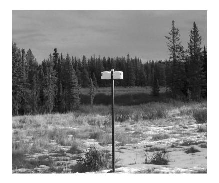
FIGURE 9. PASS multi-rain shelter installation (courtesy from PAMZ).
