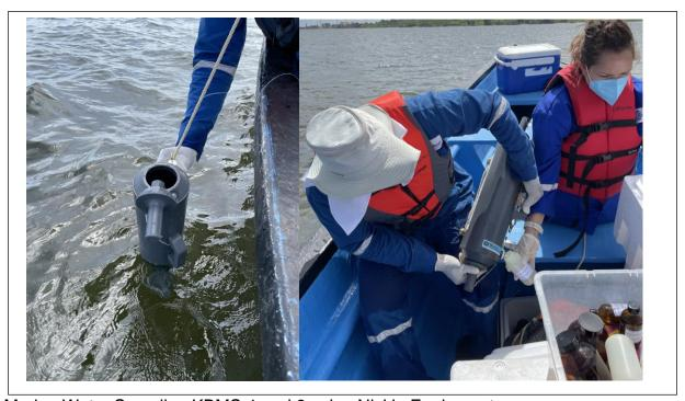
Marine Water Sampling KBMS-1 and 3 using Niskin Equipment
