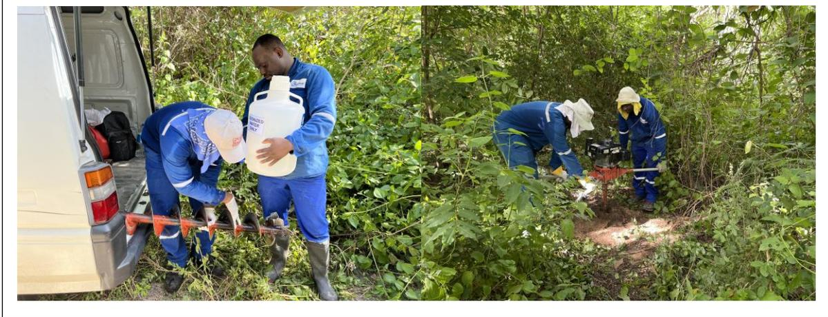
Soil Sample 6 (KBH6)- Auger Sanitization SOP and Auguring -Wash and sterilize equipment with Distilled and Deionized water after each soil sample taken.
